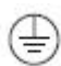
FPN Figure 250.126 One Example of a Symbol Used to Identify the Grounding Termination Point for an Equipment Grounding Conductor.
